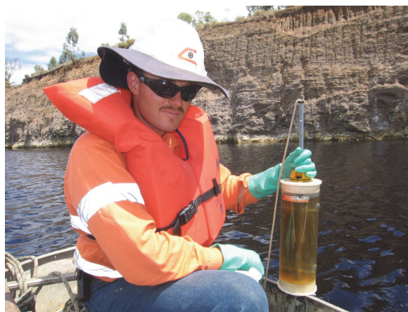
Figure 4 PPE can consist of a number of items: protection against impact, cuts and abrasions; protection from AMD waters; protection from the sun; and buoyancy aid in case of immersion in the lake (Photo courtesy of C.D. McCullough)
