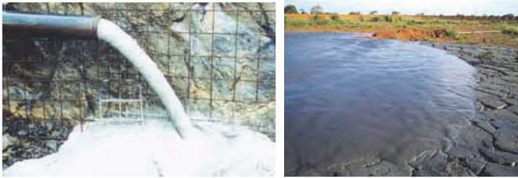
Figure 5 Cemented paste underground backfill (left), surface paste tailings disposal (right)
