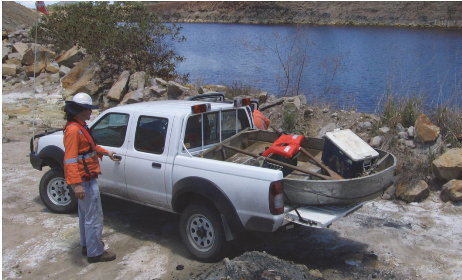
Figure 6 Loading and unloading from transport vehicles and carrying boats across rough and broken terrain is probably one of the greatest manual handling risks workers around pit lakes face (Photo courtesy of C.D. McCullough)
