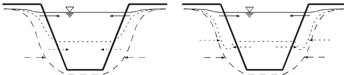
Figure 1 Interaction between pit lake and groundwater without (left), and with fast filling by diversion of river water or mine water (right), in addition to groundwater rebound. Long dash (–) water level and flow during mining, short dash (–) water level and flow during filling of pit lake, solid (—) water level and flow after establishing a new long-term hydrological balance (after Schultze et al., 2011a, simplified)
