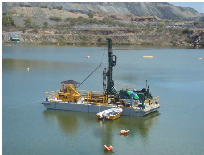
Figure 9 Investigations of in-pit tailings geochemistry, Ranger Uranium Mine, Northern Territory, Australia (Photo courtesy of Energy Resources of Australia Ltd)
