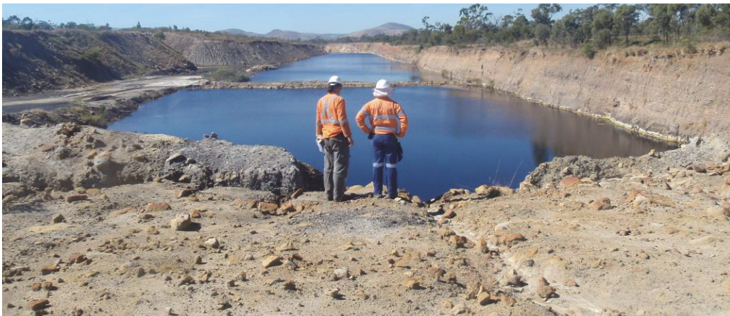
Figure 3 Misapplied, regulation can be a major obstacle to development of innovative mine water treatment and closure scenarios. Controversially for state regulators, but with strong community support, this passive treatment field experiment in North Queensland used raw sewage as a carbon source (McCullough et al., 2008) (Photo courtesy of C.D. McCullough)
