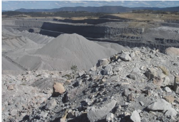
Figure 3 Progressive mining and pit backfilling, Warkworth Coal Mine, New South Wales, Australia (Photo courtesy of Panoramio, Google)
