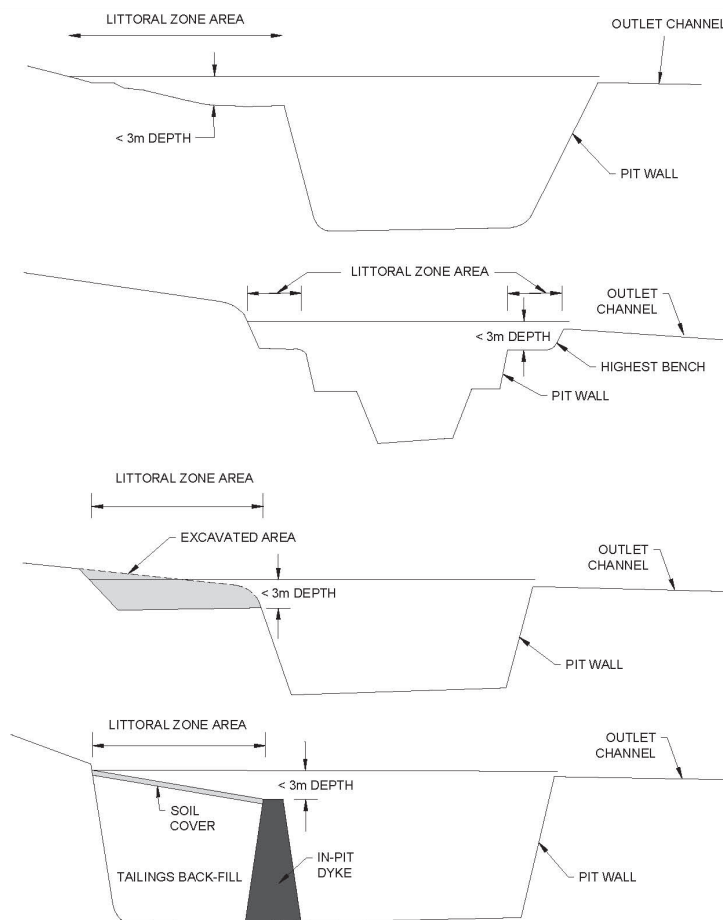
Figure 3 Methods of providing littoral zone area
