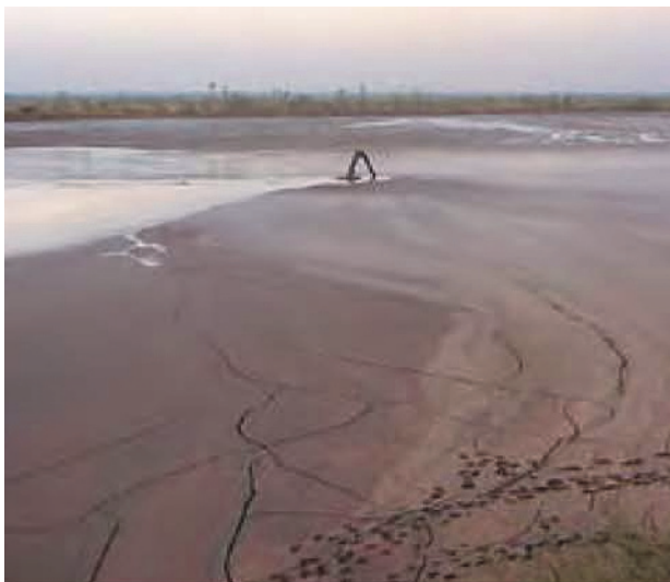
Figure 1 In-pit tailings deposition, Granites Gold Mine, Northern Territory, Australia (DITR, 2007)
